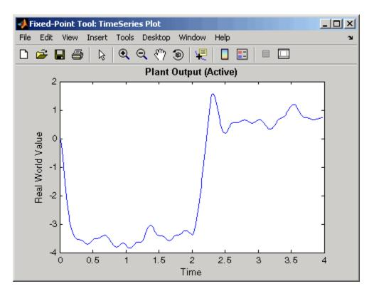
The preceding plots of the plant input and output signals reflect the initial guess at scaling. The Bode plot design sought to produce a well-behaved linear response for the closed-loop system. Clearly, the response is nonlinear. Significant quantization effects cause the nonlinear features. An important part of fixed-point design is finding a scaling that reduces quantization effects to acceptable levels.
