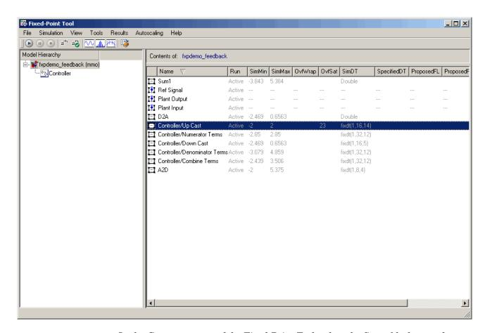
2 In the **Contents** pane of the Fixed-Point Tool, select the Scope block named Plant Input and then click the **Time Series Plot** button .
