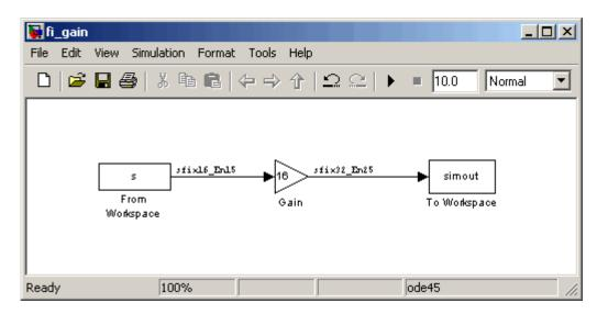
The To Workspace block writes the result of the simulation to the MATLAB workspace as a fi structure.
