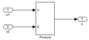
As discussed in "Fixed-Point Numbers" on page 2-3, each fixed-point quantity is calculated using its slope, bias, and stored integer. So in this example, not only is there the high-level divide called for by the block operation, but there are also intermediate additions and multiplies that are performed:
