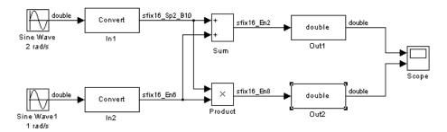
The data type display associated with the In 1 block in the model indicates that the output data type is sfix(16) (a signed, 16-bit, generalized fixed-point number) with [Slope Bias] scaling of [0.2 10]. Note that this scaling is not the block's default scaling. The data type display associated with the In 2 block indicates that the output data type is sfix(16) with binary-point-only scaling of 2^-6.
