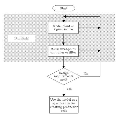
Using MATLAB, Simulink, and Simulink Fixed Point, you follow these steps of the development cycle:
