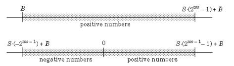
For both the signed and unsigned fixed-point numbers of any data type, the number of different bit patterns is  $2^{ws}$ .
