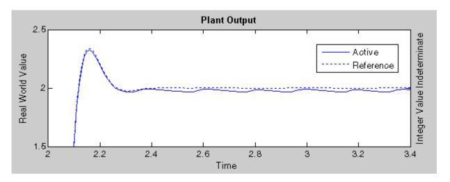
Note that the plant output signal represented by the active run achieves a steady state, but a small limit cycle is present because of poor A/D design.
