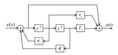
$$\frac{y(z)}{x(z)} = \frac{1 + e_i z^{-1} + f_i z^{-2}}{1 + c_i z^{-1} + d_i z^{-2}}$$
