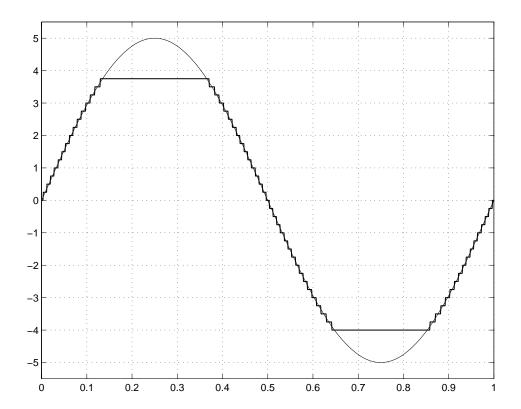
The simulation clearly demonstrates the quantization effects of fixed-point arithmetic. The combination of using a 5-bit word with a precision of  $(1/2)^2 = 0.25$  produces a discretized output that does not span the full range of the input signal.
