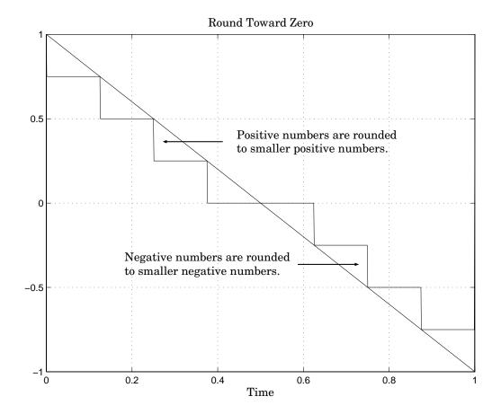
**Example: Rounding to Zero Versus Truncation.** Rounding to zero and *truncation* or *chopping* are sometimes thought to mean the same thing. However, the results produced by rounding to zero and truncation are different for unsigned and two's complement numbers.
