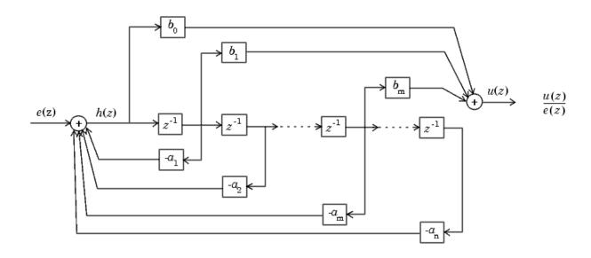
The direct form II example transfer function is given by
