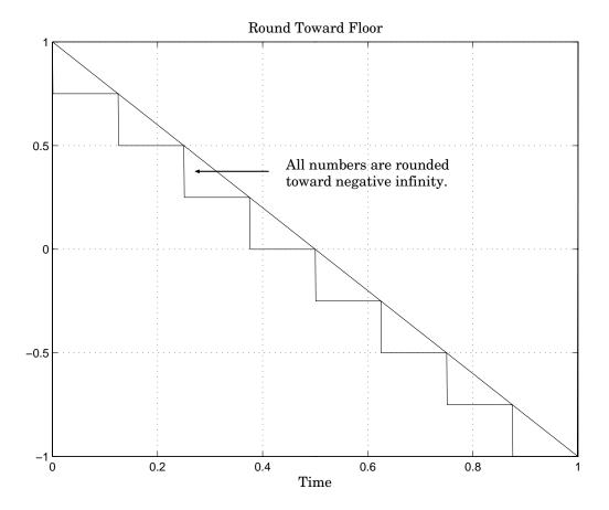
Rounding toward ceiling and rounding toward floor are sometimes useful for diagnostic purposes. For example, after a series of arithmetic operations,
